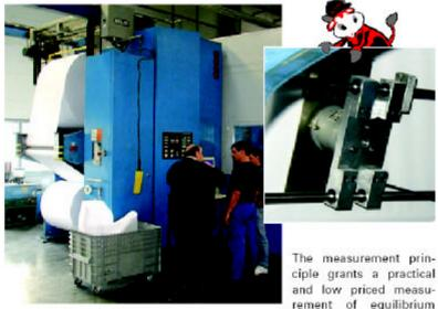
and temperature on the web, running at 500m per minute. It serves to detect and reject rolls that are out of tolerance.
