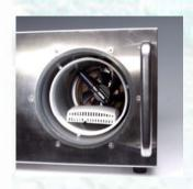
With integrated temperature control, calibrations can always be performed at a defined and constant temperature, irrespective of the ambient conditions, making the HygroGen suitable for on-site calibrations. It is also possible to calibrate equipment at its normal working temperature and humidity conditions.
